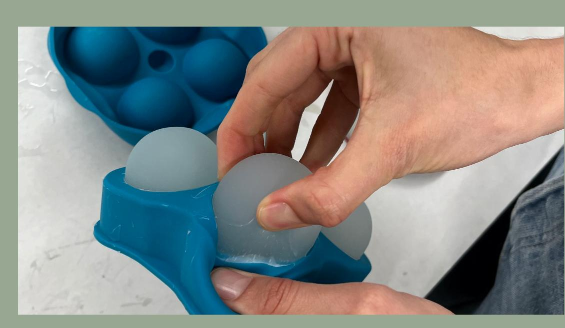
Prototype of interactive tangibles made with Ecoflex
